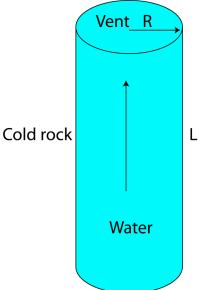
a. The radius R of the vent sets the length scale for conduction. So the conductive heat flow away from the tube is approximately
